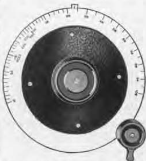
FIGURE 1. Main tuning control for the new beat-frequency oscillator
